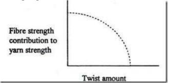
On the other hand, as yarn twist is increased, the frictional resistance between the fibres gradually increases until a point is reached at which slippage is virtually impossible. The relationship is illustrated in the diagram below:
