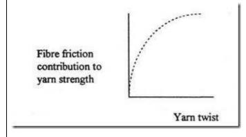
The effect of twist/spinning drum speed on the strength of dref yarns is, therefore, determined by a combination of the two effects just described above, and the resulting relationship is as illustrated in Figure 1.
