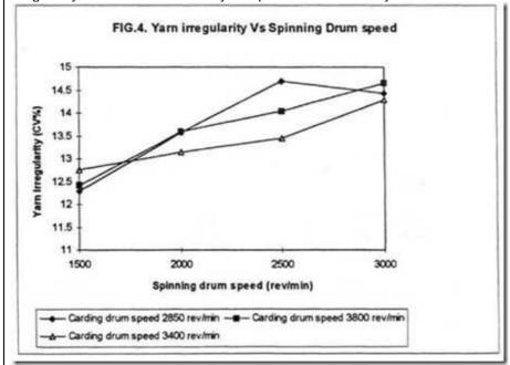
From Figure 4, it is found that when the spinning drum speed increases, the yarn irregularity (CV%) increases. Besides, the Figure shows that carding drum speed contributes little influence on the CV% value. As the spinning drum speed/twist increases, the mean yarn volume decreases, making the yarn more sensitive to the change of volume (unevenness). Thus, a higher CV% results when compared with yarns of same count, but larger volume/lower twist level.
