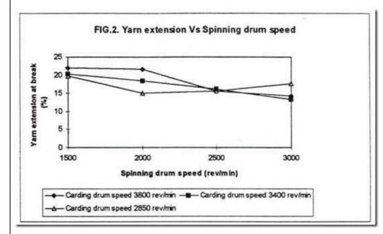
In order to explain the phenomenon, comparisons are now made on the strength and extension values between nylon filament core, Dref yam with core and Dref without core.
